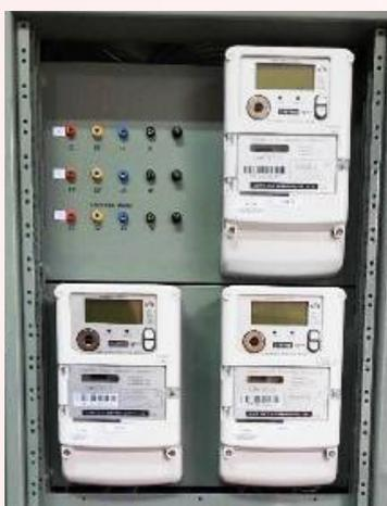
Front panel of the distribution line model designed to test voltage violations and mitigation methods
