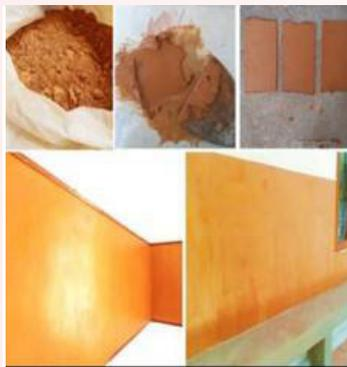
Developed soil-based wall care putty and applications
