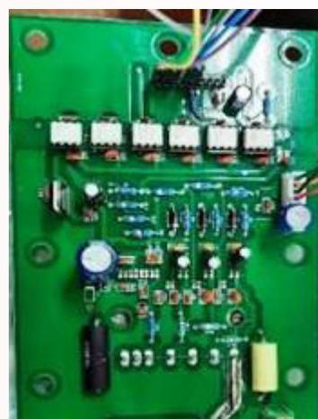
Fabricated circuit for re-phasing inverter
