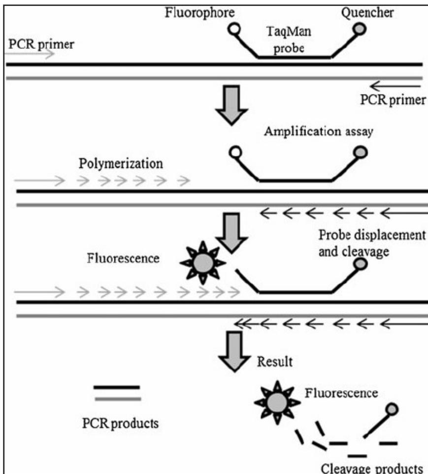
**Figure 02 : Emission of fluorescence by the fluorophore after the cleavage of the probe by DNA polymerase**
