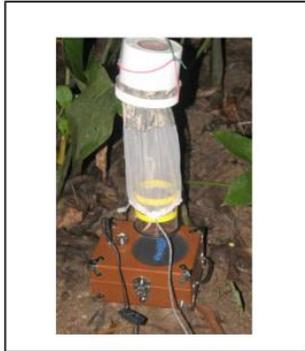
Sound trap designed to collect frog biting mosquitoes
