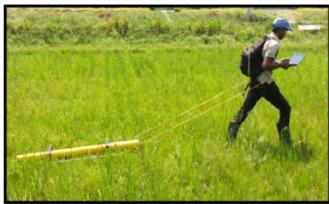
Proximal Soil Sensing of the variability of paddy grown soils
