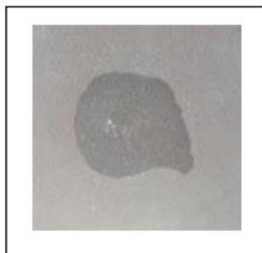
Gel polymer electrolyte hot pressed between two glass
