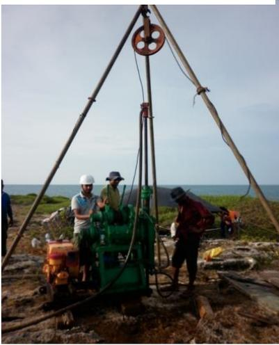
Rotary core drilling of coral and Limestone basement at Kachchativu Island
