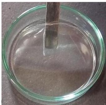
A gel polymer electrolyte prepared with solvent casting technique
