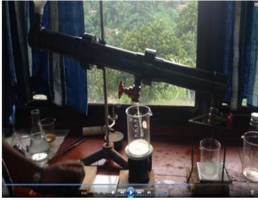
Laboratory scale reactor for the separation of service station waste oil: oil can be collected from the second compartments and water can be collected from the third compartment and membrane is fixed in the middle
