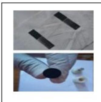
Conducting polymer electrodes used to fabricate rechargeable cells & redox capacitors
