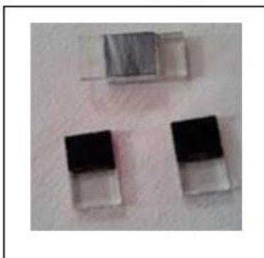
Fabricated redox capacitor
