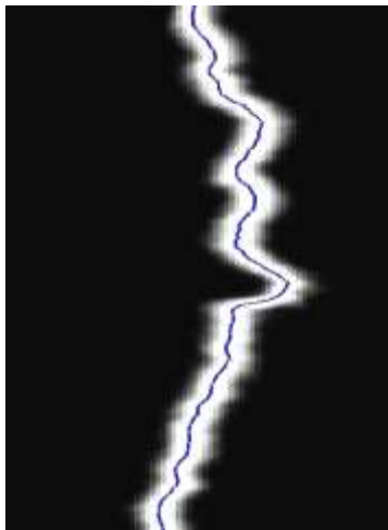
Image of a spark channel and reconstructed trajectory
