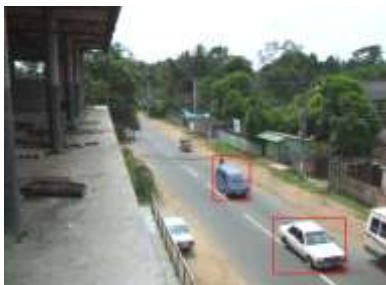
Tracking moving objects for speed detection
