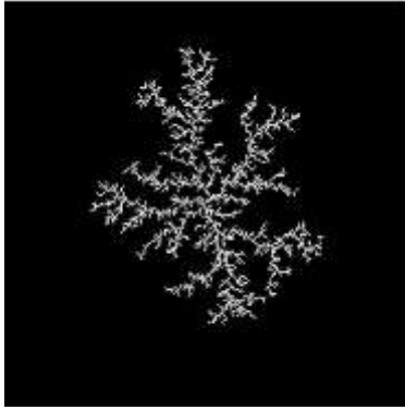
Simulated 2D radial discharge pattern
